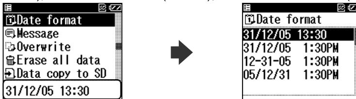
The date is displayed at the bottom of the screen using the currently selected format.
