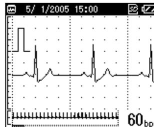
Each stored ECG data is displayed by date, time and a character representing the measurement result, refer to p. 27 for the overview of character and measurement result.
