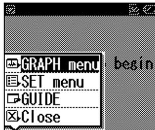
2. Select the ECG data you wish to view from the **GRAPH menu** list, then press the OK button to display the detailed view of the waveform.
