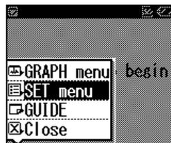
4. Press the ◀/▲ or ▼/▶ button to select the desired setting, then press the OK button to see the options for that setting.
