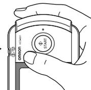
The measurement ends automatically, indicated by 4 rapid beeps.
