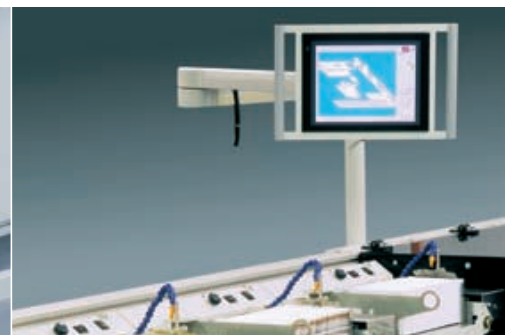
Touch screen panel NS12 - the control centre of the envelope-filling system
