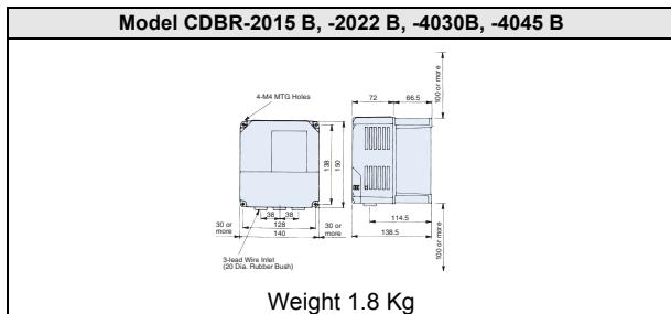
**Braking resistor unit (Inverter-mounted type)**
