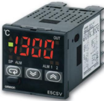
This multi-range 1/16 DIN controller with alarm function offers field-selectable PID control or ON/OFF control. The large, single display shows process value, direction of deviation from set point, output and alarm status.
