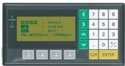
The NT11 is a Function key HMI with four text lines that can each hold up to 20 characters. It has a parallel printer connection next to a serial port for connection to a PLC. It has a LED backlight that has a life expectancy of at least 50,000 hours.
