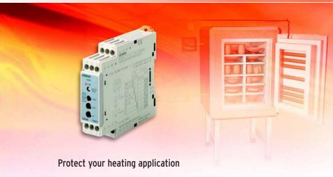
The K8AB-TH is a temperature-monitoring relay that embodies both temperature-alarm functionality and simple ON/OFF temperature control. The unit is designed specifically for monitoring abnormal temperatures to prevent excessive temperature increases and to protect equipment. It comes in a slim housing with a width of just 22.5 mm suitable for DIN-rail or direct panel mounting. Settings are selected by DIP switches, making the K8AB-TH easy to configure.
