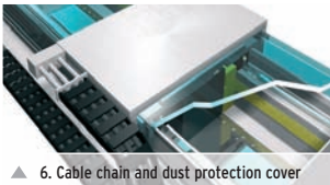
▲ 6. Cable chain and dust protection cover
