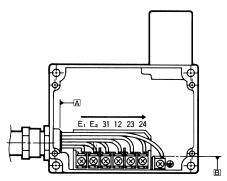
Tighten each wired terminal clockwise to a torque of 0.59 to 0.78 N·m.
