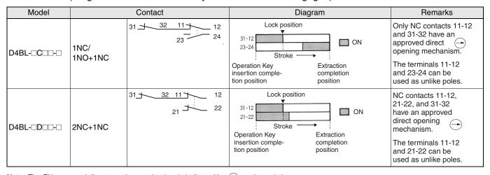
**Note:** The EN-approved direct opening mechanism is indicated by  $\longrightarrow$  on the switch.
