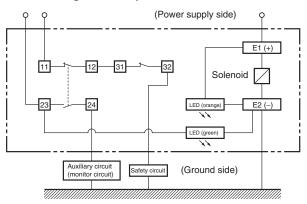
4. Orange: Lights when the solenoid turns ON. Green: Lights when power turns ON.
