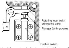
Be sure to check the mechanical lock and solenoid release functions when mounting the D4BL.
