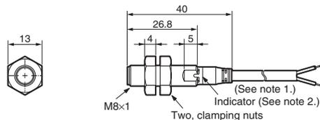
**Note 1.** 4-dia. vinyl-insulated round cable with 3 conductors (Conductor cross section: 0.3 mm<sup>2</sup>; Insulator diameter: 1.3 mm), Standard length: 2 m
