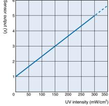
F3UV-XA + F3UV-HM + F32-300 (output characteristics at 300 mW/cm<sup>2</sup> when sensitivity is set)
