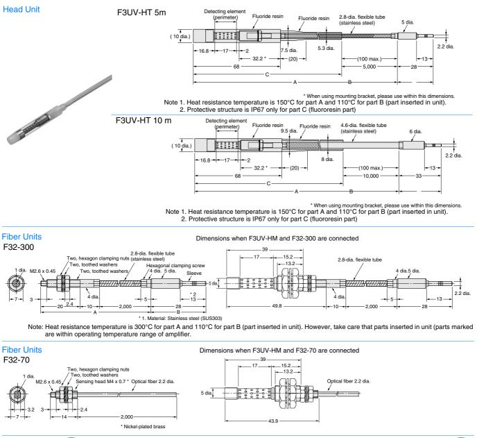
Note: free-cut indicates that free-cutting is possible. Free-cutting is not possible on units that are not marked with free-cut.
