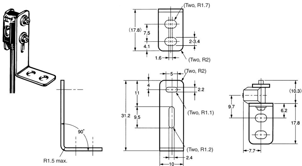
Material: 1.2-mm-thick stainless steel (SUS304)
