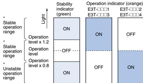
Note: If the E3T's operation level is set to the stable operation range, the E3T will be in most reliable operation without being influenced by temperature change, voltage fluctuation, dust, or setting change. If the operation level cannot be set to the stable operation range, pay attention to environmental changes while operating the E3T.
