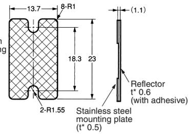
**Note:** A reflector and a stainless steel mounting plate are supplied together as a set.
