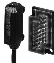
The world first coaxial Retroreflective type in this size. When used with a small reflector, this sensor completes 2 mm dia. small work detection and 200 mm sensing distance. The switch detects small works, such as IC chips on tape, and the pin-point beam makes optical axis adjustment easy, achieving stable detection.
