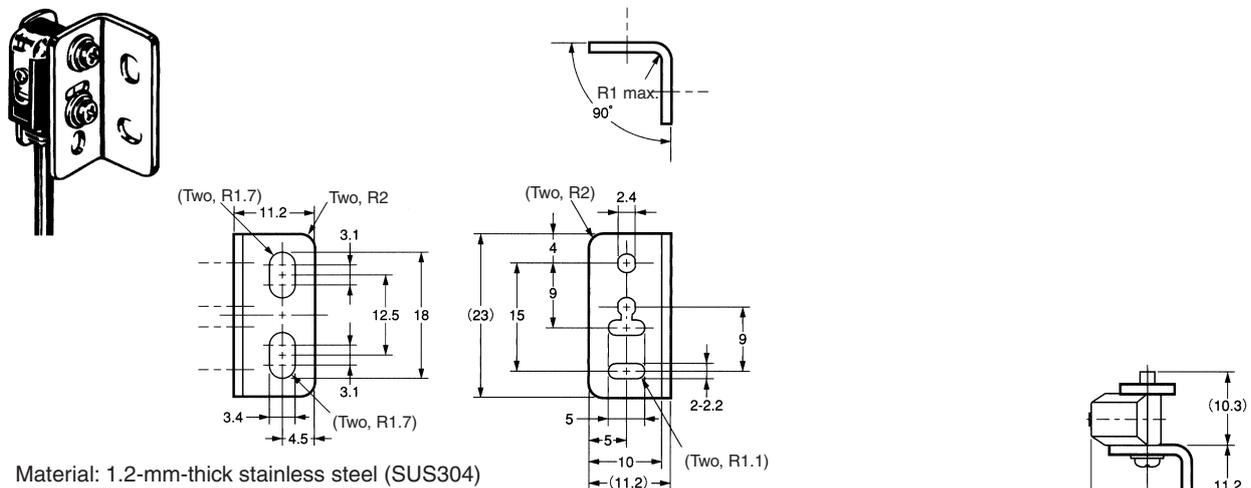
Material: 1.2-mm-thick stainless steel (SUS304)
