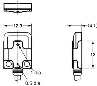
Material: 0.2-mm-thick stainless steel (SUS301)
