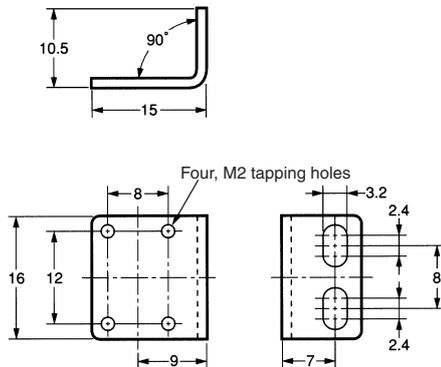
Material: 1.2-mm-thick stainless steel (SUS304)
