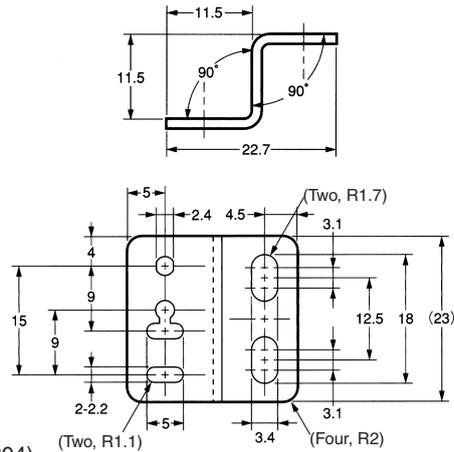
Material: 1.2-mm-thick stainless steel (SUS304)
