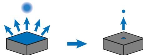
The conventional LED emits light from its surface. It has a large degree of light dispersion, increasing the loss when creating a small beam.
