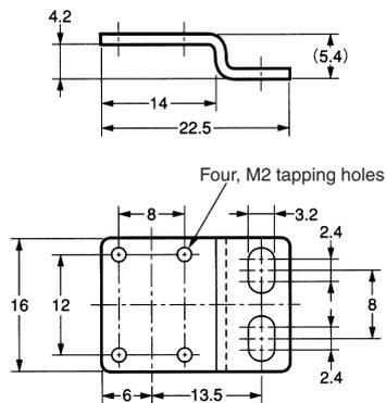
Material: 1.2-mm-thick stainless steel (SUS304)
