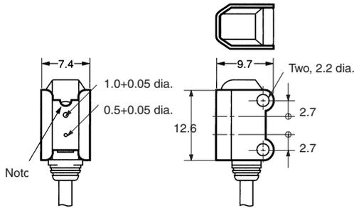
**Note:** Align the notch direction of the Slit when installing on the Emitter and Receiver.
