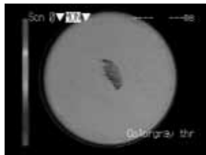
Color-grayed image Defects barely visible in the original image stand out clearly.
