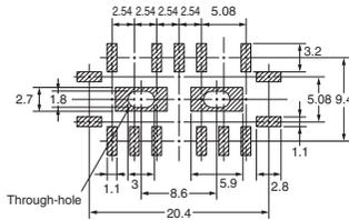
Note: Each value has a tolerance of  $\pm 0.3$  mm.
