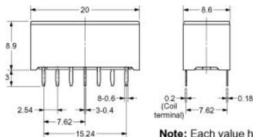
**Note:** Each value has a tolerance of  $\pm 0.3$  mm.
