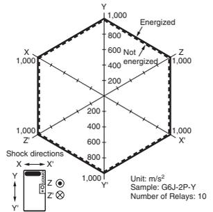
Conditions: Shock is applied in ax, ay, az directions three times each with and without energizing the relays to check the number of contact malfunctions.
