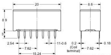
**Note:** Each value has a tolerance of  $\pm 0.3$  mm.
