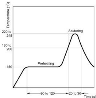
**Note:** The temperature profile indicates the temperature on the circuit board surface.
