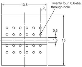
**Note:** The above compensation plate is used to measure the loss by the relay.
