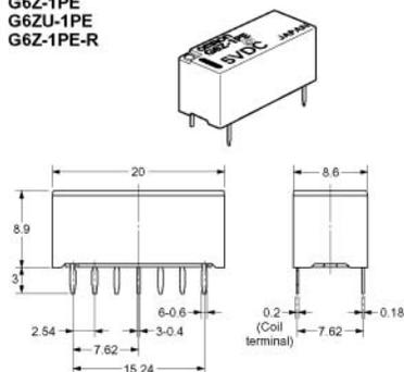
Note: Each value has a tolerance of  $\pm 0.3$  mm.
