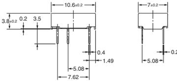
**Note:** Each value has a tolerance of  $\pm 0.3$  mm.
