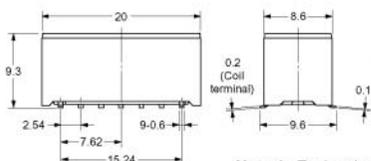
**Note 1:** Each value has a tolerance of  $\pm 0.3$  mm.
