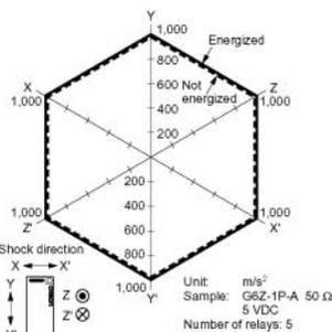
Conditions: Shock is applied in ±X, ±Y, and ±Z directions three times each with and without energizing the Relays to check for contact malfunctions.
