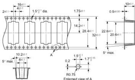
**Note:** The radius of the unmarked corner is 0.3 mm.
