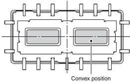
**Note:** To obtain high-frequency characteristics close to the charts shown on page ?, solder the convex point on the undersurface of the relay to the ground pattern of the substrate..
