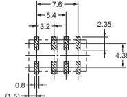
Note: Each value has a tolerance of  $\pm 0.3$  mm.
