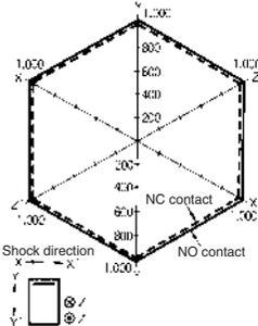
**Condition:** The Units were shocked at the rate of 500 m/s<sup>2</sup> three times each in the X, Y, and Z directions with and without voltage imposed on the Units until the Units malfunctioned.
