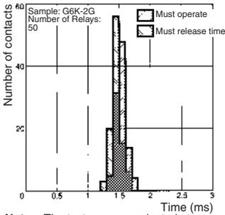
**Must Operate and Must Release Bounce Time Distribution (see note)**
