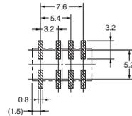
Note: Each value has a tolerance of  $\pm 0.3$  mm.
