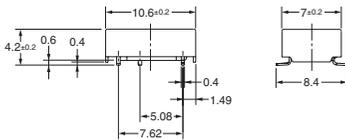
**Note:** Each value has a tolerance of  $\pm 0.3$  mm.
