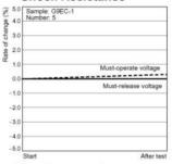
Characteristics were measured after applying a shock of 490 m²/s to the test piece 3 times each in 6 directions along 3 axes. The percentage rate of change is the average value for all of the samples.
