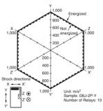
Conditions: Shock is applied in  $\pm x$ ,  $\pm y$ ,  $\pm z$  directions three times each with and without energizing the relays to check the number of contact malfunctions.
