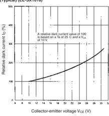
Figure 12. Dark Current Imposed Voltage Dependency (Typical) (EE-SM3B)
