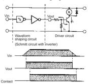
If the Schmitt trigger circuit is configured of transistors, a residual voltage may exist in the output of the circuit. Therefore, confirm that the rated voltage is present across the relay coil, or that the residual voltage drops to zero when the relay releases. When an IC (e.g., TC74HC132P) is used, this value is close to zero.
