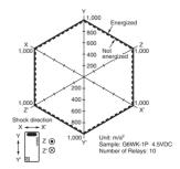
Conditions: Shock is applied in  $\pm X$ ,  $\pm Y$ , and  $\pm Z$  directions three times each with and without energizing the Relays to check the number of contact malfunctions.
