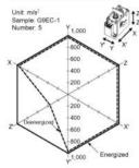
The value at which malfunction occurred was measured after applying shock to the test piece 3 times each in 6 directions along 3 axes.
