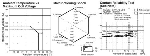
Note: The maximum coil voltage refers to the maximum value in a varying range of operating power voltage, not a continuous voltage. Quantity Tested: 10 Units Test Method: Shock was a
