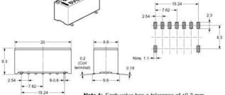
Note 1: Each value has a tolerance of ±0.3 mm.
