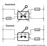
Even in a "correct" circuit, note that the insulation performance of the switch may deteriorate and the switch life may be shortened because one load is connected to one contact.
