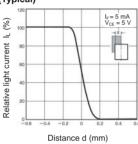
EE-SX1109 Sensing Position Characteristics (Typical)
