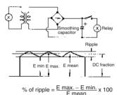
E max.: Max. ripple E min.: Min. ripple E mean: Mean DC value
