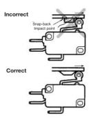
Make sure that no improper load is imposed on the actuator, otherwise the actuator may incur local abrasion. As a result, the actuator may become damaged or its life expectancy shortened.
