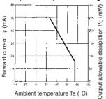
LED Current vs. Ambient Temperature Characteristics (Typical)
