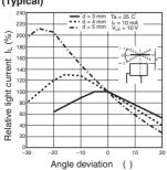
Sensing Angle Characteristics (Typical)
