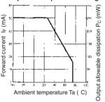
LED Current vs. Ambient Temperature Characteristics (Typical)
