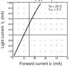
EE-SX1109 Light Current vs. Forward Current Characteristics (Typical)
