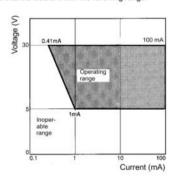
Minimum operating load 1 mA at 5 VDC
