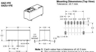
2: The coplanarity of the terminals is 0.1 mm max.
