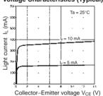
EE-SX1108/1131 Light Current vs. Collector–Emitter Voltage Characteristics (Typical)
