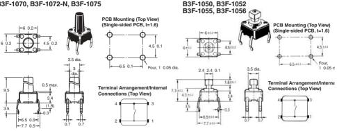
Horizontal, Projected Plunger Type (with Ground Terminal)
