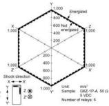
Conditions: Shock is applied in ±X, ±Y, and ±Z directions three times each with and without energizing the Relays to check for contact malfunctions.
