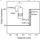
Repetitive Sensing Position Characteristics (in vertical direction, typical)
