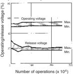
With OMRON's MA415A Contactor (40 mA at 200 VAC)
