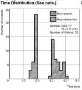
Must Operate and Must Release Bounce Time Distribution (See note.)
