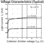
EE-SX1109 Light Current vs. Collector-Emitter Voltage Characteristics (Typical)
