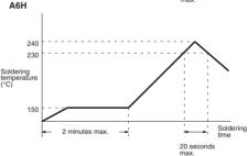
Do not use reflow soldering for any models other than the A6S and A6H. Otherwise the plastic case may melt or deform.
