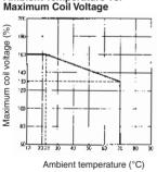
The maximum coil voltage refers to the maximum value in a varying range of operating power voltage, not a continuous voltage. Note:
