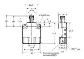
Note: NC-OFF: The force applied to the actuator to cause it to move from the free position to the position at which the NC contact opens.
