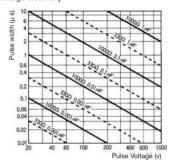
Note: For low-voltage models, sufficient voltage may not be applied to the SSR because of the relationship between C, R, and the internal impedance. When deciding on a value for R, check the input impedance for the SSR.
