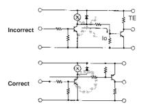
A circuit that produces a control output as soon as the relay operates must be carefully designed. In the example on the left, electrode dark current flows as shown when the relay operates. When dark current flows into the relay coil, the relay's resistivity to shock and vibration may degrade.
