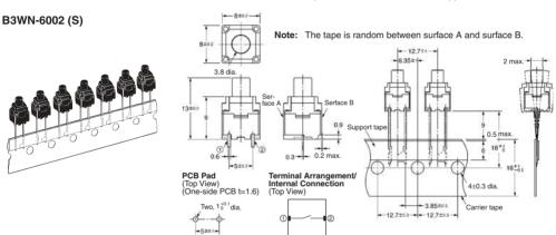
Note: Switch fixing direction (A and B) on the tape may change.
