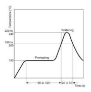
Note: The temperature profile indicates the temperature on the circuit board surface.
