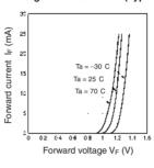
LED Current vs. Supply Voltage (Typical)
