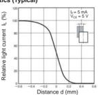
EE-SX1131 Sensing Position Characteristics (Typical)
