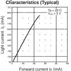
EE-SX1108/1131 Light Current vs. Forward Current Characteristics (Typical)
