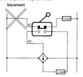
Do not configure a circuit that may place a voltage between the contacts of the Switch; otherwise metal deposition will occur between the contacts.
