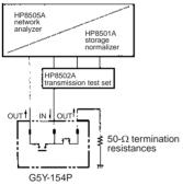
The following characteristics are measured with contacts unrelated to the measurement terminated at  $50\Omega$ , when a signal is applied from input terminal 11 to output terminal 8 or from input terminal 11 to output terminal 11 to output terminal 12 of the sample.
