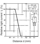
Sensing Position Characteristics (EE-SH3-C(S))
