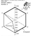
The value at which malfunction occurred was measured after applying shock to the test piece 3 times each in 6 directions along 3 axes.
