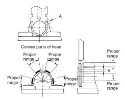
Refer to the following to adjust the stroke of the lever based on the mounting hole level.
