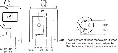
Note 1. "Lights when operated" means that when the actuator is turned or pushed and the Limit Switch contact leaves the NC side, the indicator lights.
