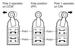
Pole 1 operates on CW and pole 2 operates CCW.
