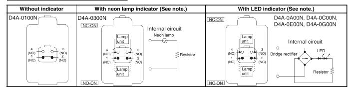
Note: Indicator setting is made before shipping so that it will light when the Limit Switch is not being operated.
