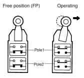
Pole 1 and pole 2 are actuated simultaneously. Operates either CW, CCW, or both.
