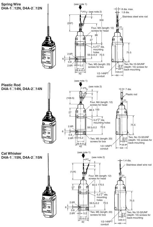
Note: 1. The stainless rod can be operated from any direction except the axial direction (i.e., from the top).
