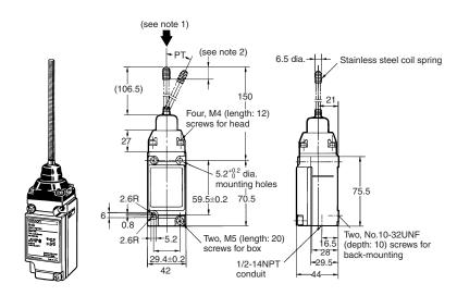
Note: 1. The stainless rod can be operated from any direction except the axial direction (i.e., from the top).
