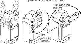
There are four kinds of fork lever locks. The position of each roller is different. It is possible to use D4A-E00 through D4A-E30 levers instead, if they are reversed before attaching. They can be used with D4A-□□05N models only.
