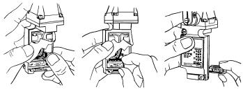
Push the claw securing the lamp section to the right (do not push strongly).
