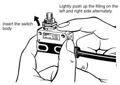
Be sure that the clamp is inserted to the full depth, because the Switch will not function properly if one of the clamps is improperly inserted.
