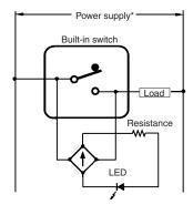
Note: \*An external 24VDC power supply can be used, eg. OMRON S8VS.
