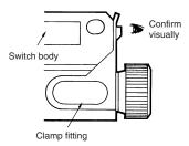
If the clamp is properly inserted up to the full depth, it will not slide out easily. Be sure to carefully confirm all the above items.
