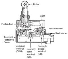
Note: M4 binding head screws (with toothed washers) are used as the terminal screws.
