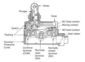
Note: M4 binding head screws (with toothed washers) are used as the terminal screws.
