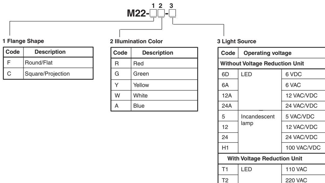
**Note:** The LED lamp (24 VAC/VDC) can be lit by directly applying 110 VAC/VDC (220 VAC/VDC) to the lamp terminal. LED incorporates the 24-VAC/VDC type.
