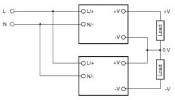
Depending on the model, internal circuits may be damaged due to startup failure when the power is turned ON if loads such as a servomotor or operational amplifier may operate in series.
