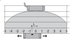
5 mm misalignment tolerance after setting
