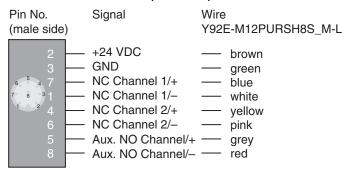
Note: For 2NC+1NO contact configuration models (F3S-TGR-N□□C-21-□□), if the auxiliary circuit is not fitted or used, then cut and discard the brown/orange or the grey/red conductors.
