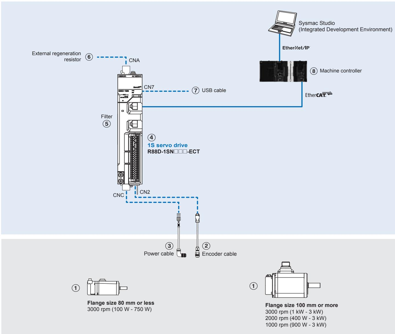
Servo motors, power & encoder cables
