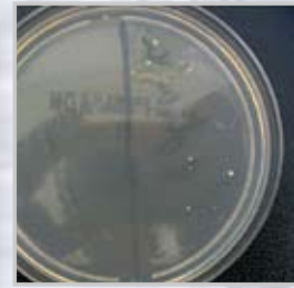
Active bacteria reduction on E2F-D housing after 12 hours.
