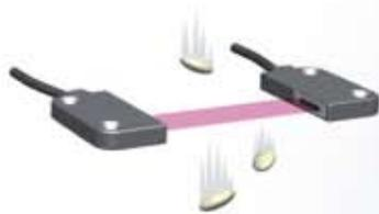
The E3X-NA-F detects objects extremely quickly: it needs no more than 20  $\mu$ s. It reliably detects falling SMD components or small metal parts. It can also be used for mark sensing or for determining speeds.
