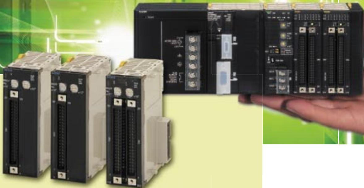
For Point-to-Point (PTP) applications the CJ1W-NC range combined with the CJ1 PLC offers the best performance/size ratio on the market. There are 3 models with 1, 2 or 4 axes capability, with the ability to handle up to 100 positions and a pulse rate of 500kbps.
