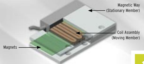
▲ Coreless GW linear motors construction results in zero-attraction force and zero-cogging.
