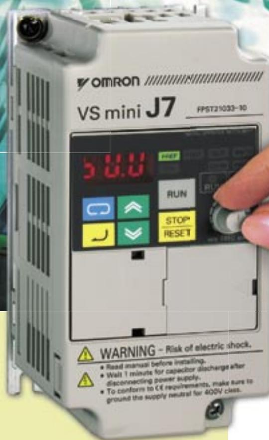
Simplicity and cost effectiveness are the key design features for the J7. Using Volts/Frequency control with on-line torque compensation the drive provides 100% torque down to 1.5Hz. The J7 has a built-in speed setting potentiometer, 4 configurable inputs, one configurable relay output as well as a multi-function analogue output.
