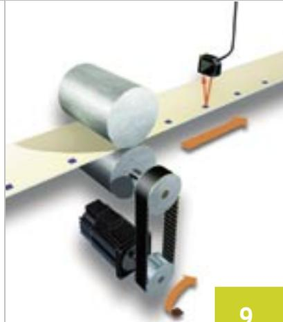
▶ A high-precision positioning system can be constructed to meet a broad range of applications by combining the Position Control Unit with a high-speed, high-precision Omron servo motor and servo driver.
