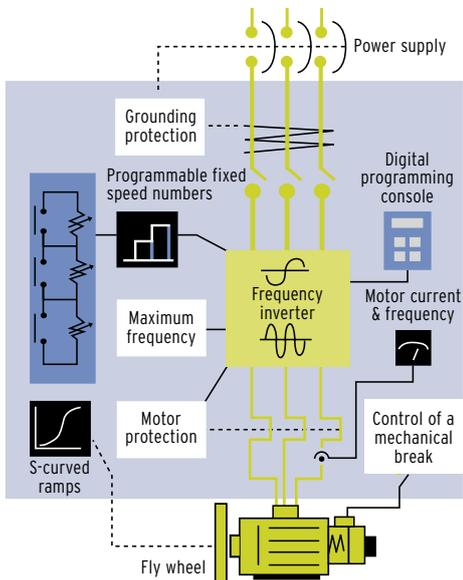
▼ Inverter J7 controls the speed and positioning of a car wash station.
