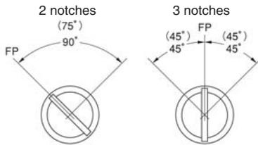
**Note:** 1. The angles in parentheses are for automatic-reset models.
