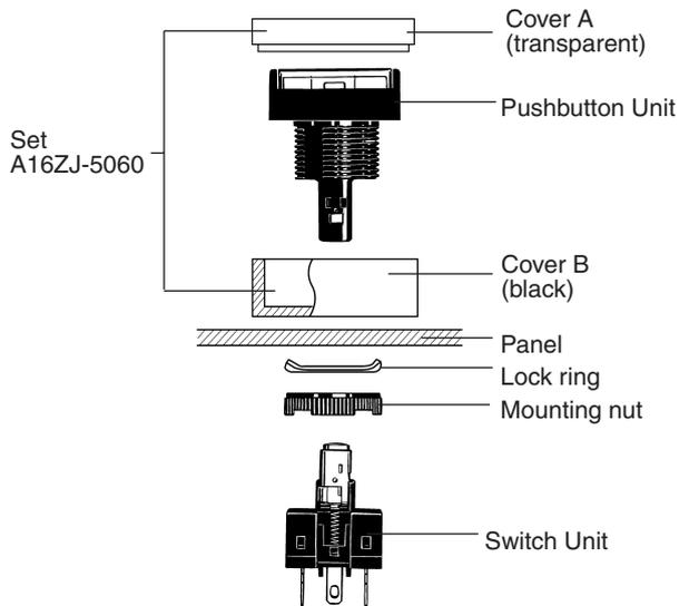
1. Separate the Dust Cover into 2 parts: cover A and cover B.
