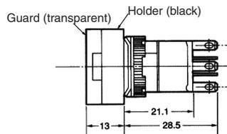
**Note:** The above illustration shows the case where 4.5 mm is provided for the distance "x." If no clearance is required for the "x" section, the vertical mounting dimension can be as small as 24 mm. Set this distance according to operating conditions. For models with PCB terminals, the horizontal mounting dimension is 24 mm min.
