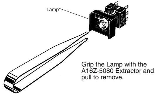
Grip the Lamp with the A16Z-5080 Extractor and pull to remove.
