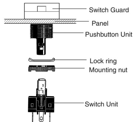
1. Insert the Case into the Switch Guard.
