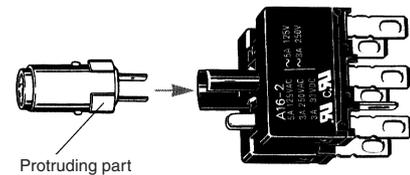
The Lamp can be mounted from the Pushbutton end by using the A16Z-5080 Extractor. The lamp can be mounted by following the opposite procedure for removing the Lamp.
