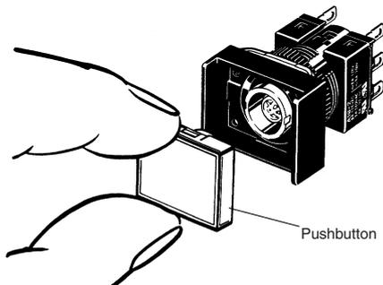
2. To attach the Pushbutton, push until it clicks into place.
