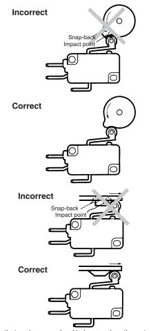
· Make sure that no improper load is imposed on the actuator, otherwise the actuator may incur local abrasion. As a result, the actuator may become damaged or its life expectancy shortened.
