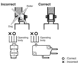
· Make sure that the operating body moves in a direction where the actuator moves. If the actuator is a pin plunger type, make sure that the operating body presses the pin plunger vertically.
