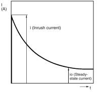
The switching capacity of each Switch appearing on a datasheet is the rated capacity. When applying the Switch to a circuit with a special load with unusual inrush and switching current and voltage waveforms, be sure to test the Switch under the actual conditions before use.
