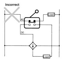
Do not configure a circuit that may place a voltage between the contacts of the Switch; otherwise metal deposition will occur between the contacts.
