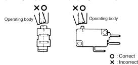
Operate the actuator of a hinge roller lever or simulated hinge lever type in the direction shown below. Operating the actuator in the opposite direction may result in deformation of the lever.
