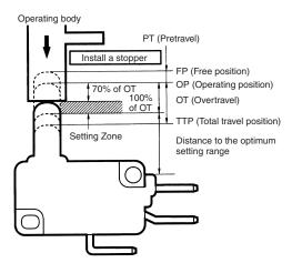
If the stroke is set in the vicinity of the operating position (OP) or at the releasing position (RP), switching operation may become unstable. As a result, the Switch cannot ensure high reliability. Furthermore, the Switch may malfunction due to vibration or shock.
