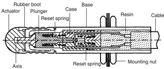
**Note:** NBR rubber is used with this Switch.
