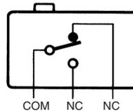
**Note:** With the reverse-type models (X-10GM□), the NC and NO terminal arrangements are reversed.
