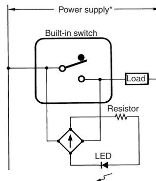
\*An external power supply can be used, eg. OMRON S8VS or S82K.
