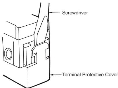
When mounting the Terminal Protective Cover to the case, align the cover on the case and then press the cover down to mount it firmly. If the cover is pressed down in an inclined position, rubber packing will deform and thus affect the sealing capability.
