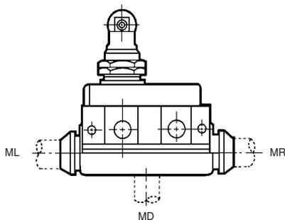
**Note:** Three leads (COM, NO, and NC) are provided for terminal connections.
