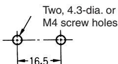
When mounting the panel mount type (SHL-Q55, SHL-Q2255, or SHL-Q2155) on a panel, tighten the hexagonal nuts of the actuator to a torque less than 7.84 N·m.
