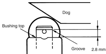
To allow the roller lever-type actuator to travel properly, adjust the dog and cam so that the arrow head is positioned between the two convex markers as shown below.
