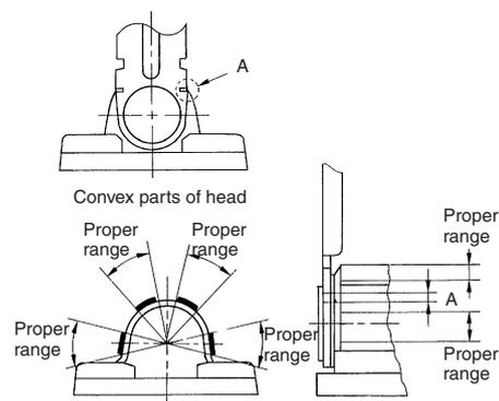
Refer to the following to adjust the stroke of the lever based on the mounting hole level.
