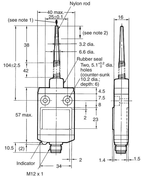
**Note:** 1. Operation is possible in any direction except parallel to the axis ↓.
