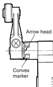
Properly adjust the stroke of the center roller lever along with the dog or cam so that the concave part (A) of the head is located between the convex parts of the head as shown below when the center roller lever is pressed by the dog or cam.
