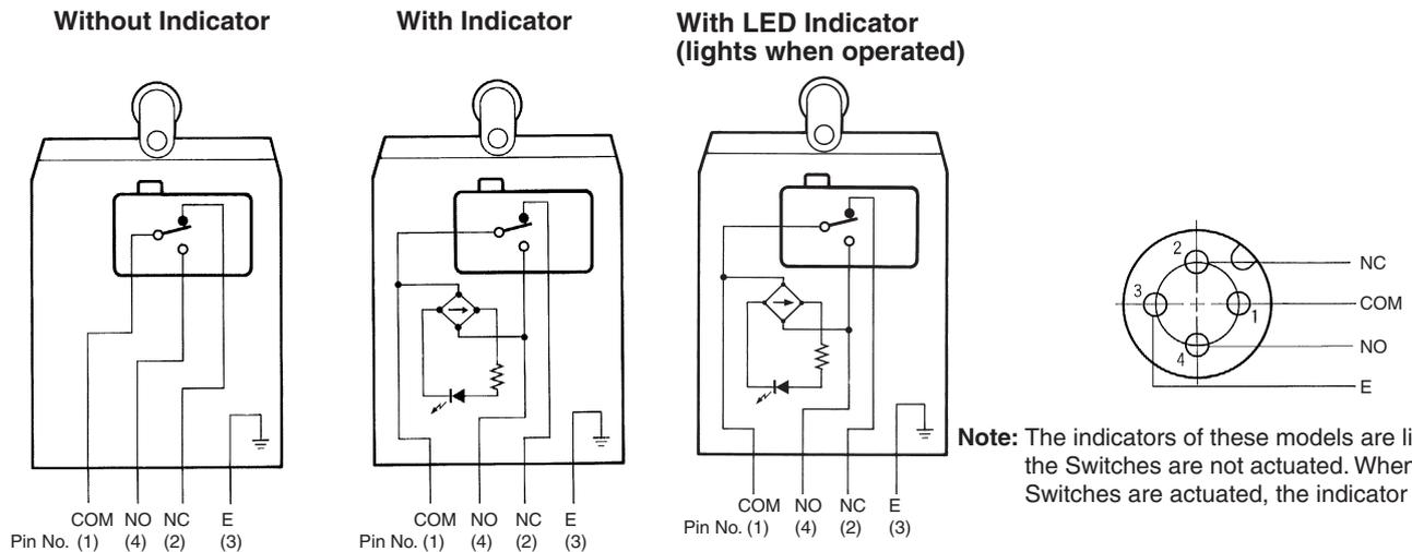
**Note 1.** "Lights when operated" means that when the actuator is turned or pushed and the Limit Switch contact leaves the NC side, the indicator lights.
