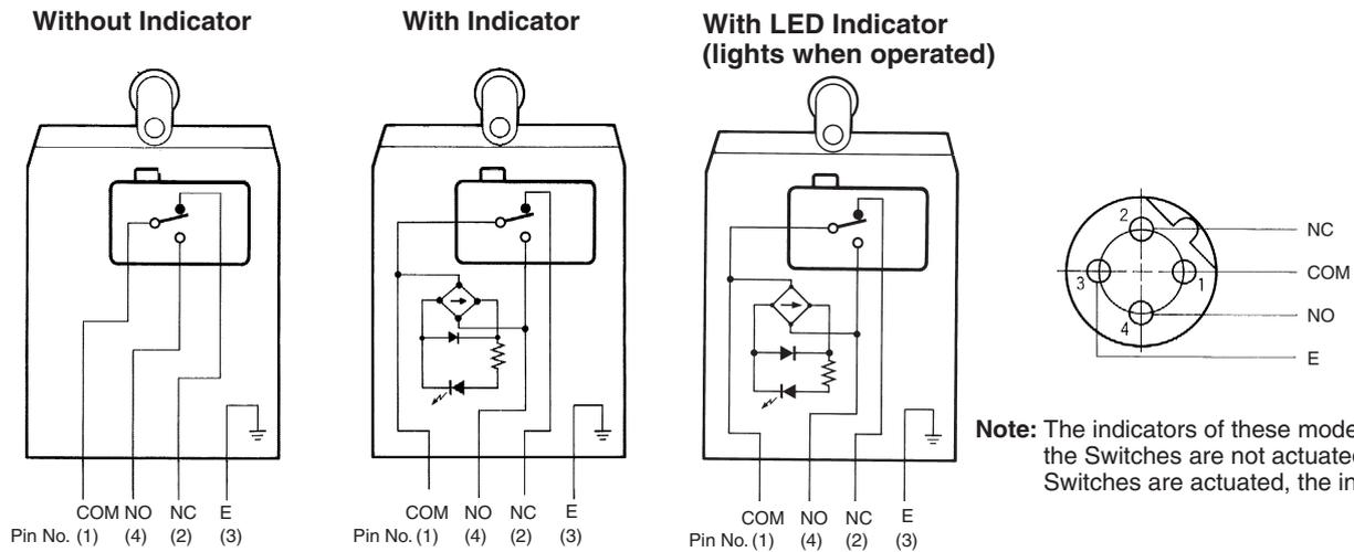
**Note 1.** "Lights when operated" means that when the actuator is turned or pushed and the Limit Switch contact leaves the NC side, the indicator lights.
