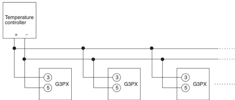
3. A Temperature Controller (with a relay output) is used to vary the duty of G3PX.
