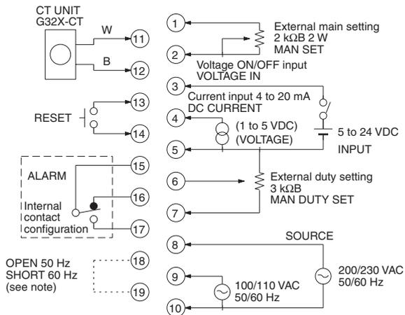
**Note:** Open the terminals for 50 Hz or short-circuit the terminals for 60 Hz. When the product is shipped, the terminals are short-circuited using a short-circuiting bar to set to 60 Hz. When using at 50 Hz, remove the short-circuiting bar.
