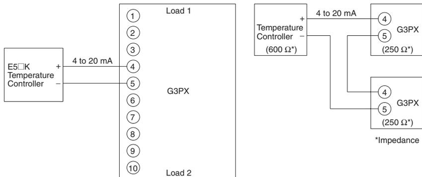
**Note:** Two G3PX models can be connected in series to OMRON's single Temperature Controller (with an internal impedance of 600 Ω) with a current output.
