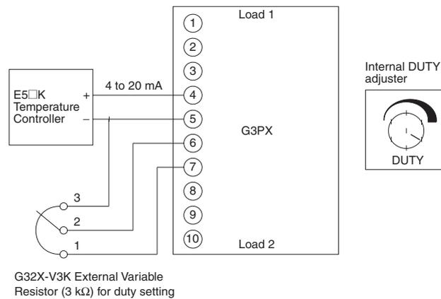
**Note:** You can change the duty with the external or internal ramp adjuster.
