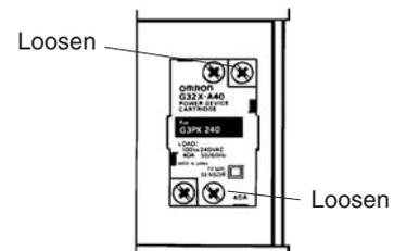
4. Loosen the screws on both corners.
