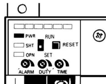
3. Adjust the sensitivity. Turn the ALARM adjuster and set to the position where the OPEN indicator is lit. Stop turning the ALARM adjuster as soon as the indicator is lit to complete the setting.
