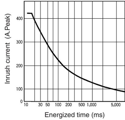
**Note:** The above are possible on condition that the G3PX is in non-repetitive operation. If the G3PX is in repetitive operation, reduce the applied current to half.
