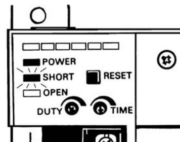
**Note:** When the G3PX detects a short-mode failure, all LEDs of the Level indicator and red SHORT indicator are lit. When you use a breaker to disconnect the load with the relay output, all LEDs of the Level indicator will be OFF regardless of the input to the G3PX.
