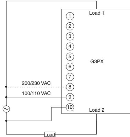
**Note:** Use a single power supply for the G3PX and the load.
