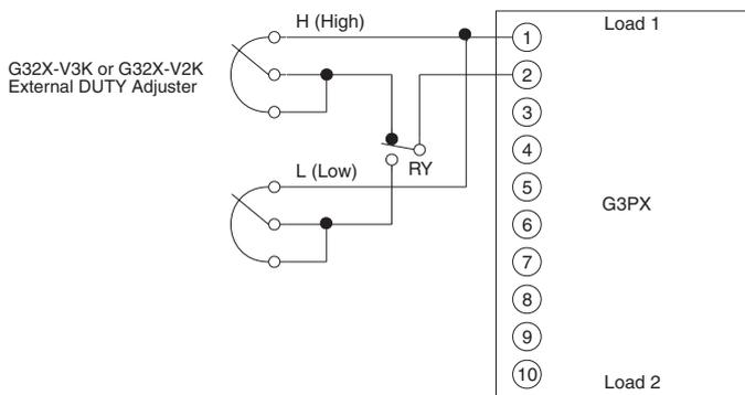
**Note:** 1. A temperature controller with relay output or a single relay can be used with the G3PX in two-position (high-and low-position) control, in which case the relay contact current is 30 mA at 12 VDC with the External DUTY Adjuster set to 0 Ω.
