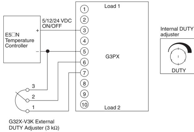
**Note:** You can change the duty with the external or internal variable resistor.
