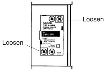
3. Insert the Cartridge into the opening of the G3PX so that the letters on the Cartridge and those on the G3PX are in the same direction and sides A and B are even.
