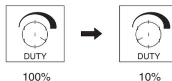
If the External DUTY Adjuster is used, set the Internal DUTY Adjuster to 100%.
