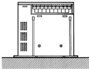
**Note:** In the case of flat mounting, the 30% derating of the load current is required.
