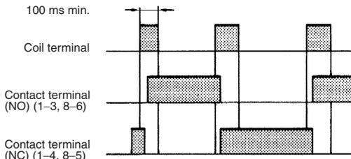
**Note:** When a pulse for application to the coil is used, such a pulse should have a width of 100 ms or more. If a pulse is applied with a width less than the operate time, the cam may fail to rotate fully.
