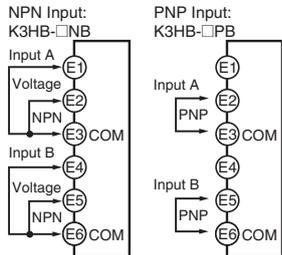
Note: E3 and E6, as well as B6, are internally connected.
