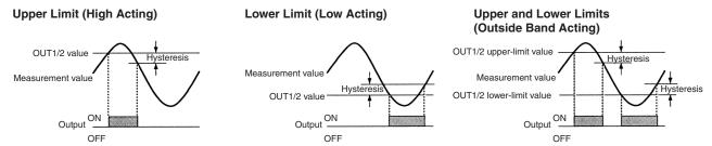
The three types of output operations shown above can be combined as desired. The following are examples of possible combinations.
