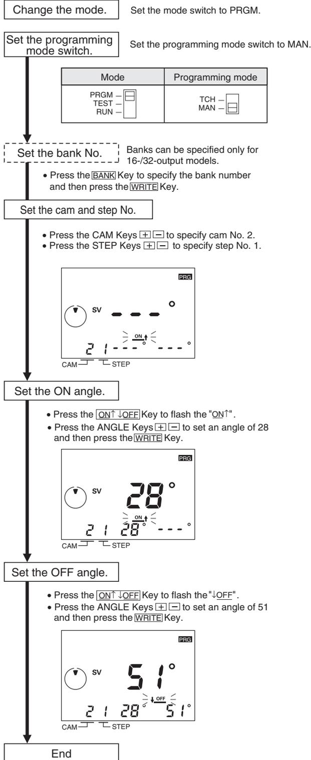
**Note:** Pressing the [↑] or [↓] Key continually will automatically increment or decrement the value. Pressing the other key during automatic increment or decrement will increase the speed.
