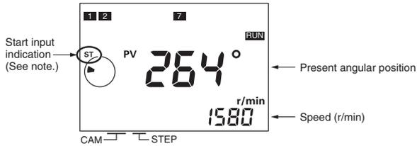
**Note:** For 16/32-output models, be sure that the start input is ON and that the start input indicator is lit. Outputs (including the cam, pulse, and run outputs) will not function if the start input is OFF. The 8-output models do not have a start input.
