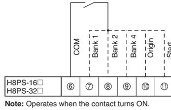
Voltage-output sensors can also be connected.
