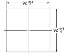
Note: Mounting panel thickness must be 1 to 5 mm.
