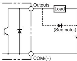
**Note:** Always connect a diode to absorb counter-electromotive force when connecting an inductive load.
