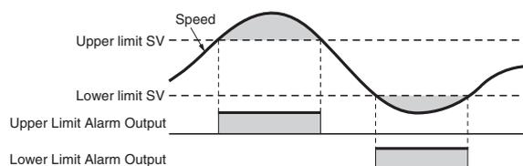
The speed alarm outputs are assigned to cam outputs as shown in the following table. The speed alarms are set to “- -” for the default settings, i.e., the normal cam outputs are enabled. If a speed alarm is set to any value but “- -”, the normal cam output for the corresponding cam number will be disabled.
