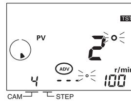
5. Set the ADV value to 2 with the ANGLE Keys  $\left[ \begin{smallmatrix} + \\ - \end{smallmatrix} \right]$ .
