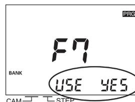
Enable or disable the bank function with the ANGLE Keys (+) (-).
