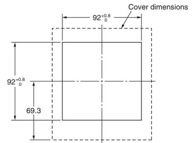
Use for flush mounting when waterproofing is required. The Y96A-96N conforms to IP66 and NEMA4 (for indoor use) standards for waterproofing. The operating environment may cause the waterproof packing to deteriorate, shrink, or harden. Therefore, it is recommended that the packing be replaced regularly.
