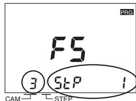
Set the cam number to 3 with the CAM Keys (+) (-) and set the maximum number of steps to 1 with the Angle Keys (+) (-). Press the WRITE Key to write the setting to memory.
