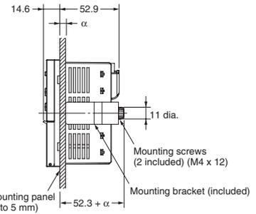
Note: An 8-output Model is shown in the above diagrams. The Encoder is connected from the bottom with 16-/32-output Models.
