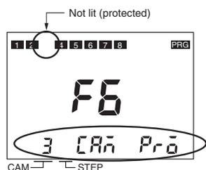
Set the cam number to be protected (and not displayed) to 3 with the CAM Keys (+) (-) and then press the WRITE Key. The output display will go out.
