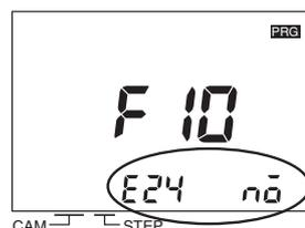
Enable or disable E24 detection with the ANGLE Keys .
