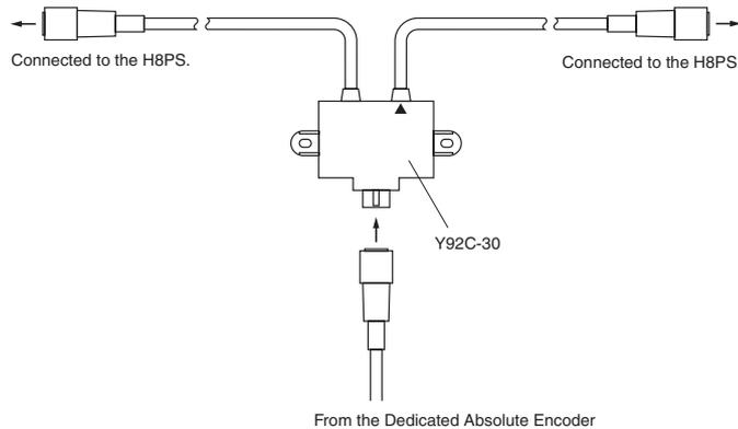
Use the cable marked with a triangle when connecting only one H8PS Cam Positioner to the Parallel Input Adapter.
