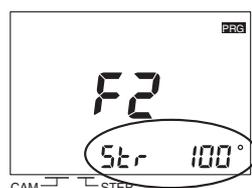
Set the pulse output start angle to 100 with the ANGLE Keys  $\left[ \right]$  and then press the **WRITE** Key.
