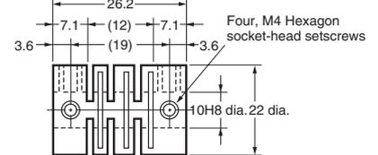
**Note:** The material is fiber-glass-reinforced polybutylene terephthalate resin (PBT).
