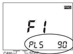
Set the number of pulses with the ANGLE Keys  $\left[ \right]$  and then press the **WRITE** Key.
