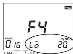
Set the upper limit set value to 20 with the ANGLE Keys  $\left[ \right]$  and then press the **WRITE** Key.
