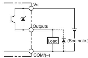
**Note:** Always connect a diode to absorb counter-electromotive force when connecting an inductive load.
