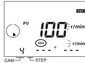
4. Set the speed to 100 with the ANGLE Keys  $\left[ \begin{smallmatrix} + \\ - \end{smallmatrix} \right]$  and then press the  $\left[ \text{WRITE} \right]$  Key.
