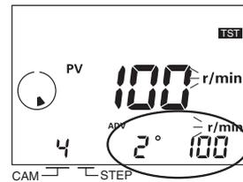
6. Press the  $\left[ \text{WRITE} \right]$  Key to write the settings to memory.
