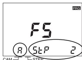
Set the cam number to 3 with the CAM Keys (+) (-) and set the maximum number of steps to 2 with the Angle Keys (+) (-). Press the WRITE Key to write the setting to memory.
