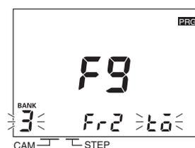
Set bank number 3 (the copy destination) with the **BANK** Key and then press the **WRITE** Key.
