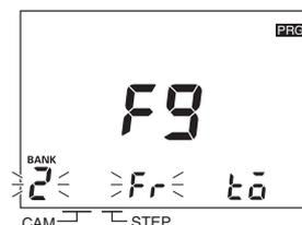
Set bank number 2 (the copy source) with the **BANK** Key and then press the **WRITE** Key.
