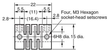
**Note:** The material is fiber-glass-reinforced polybutylene terephthalate resin (PBT).
