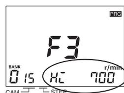
Set the upper limit set value to 700 with the ANGLE Keys  $\left[ \right]$  and then press the **WRITE** Key. (See note.)
