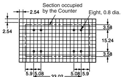
Note: Processing dimensions are for 28-pin IC socket.
