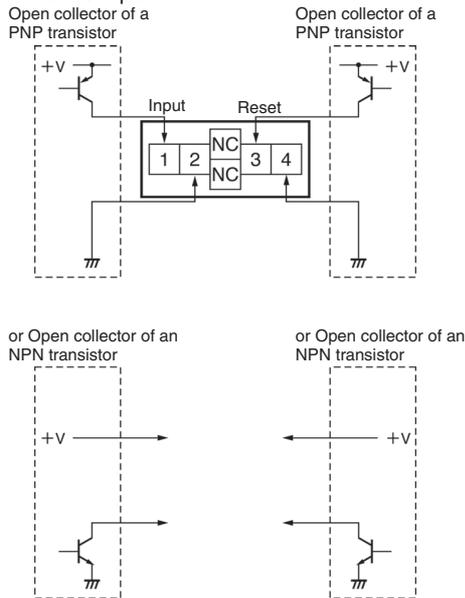
**Note:** 1. Terminals 2 and 4 (input circuit and reset circuit) are functionally isolated.
