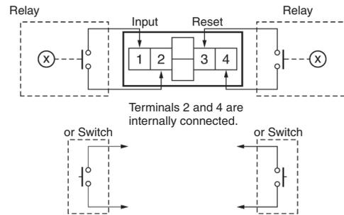
**Note:** Use Relays and Switches that have high contact reliability because the current flowing from terminals 1 or 3 is small. It is recommended that OMRON's G3TA-IA/ID be used as the SSR.
