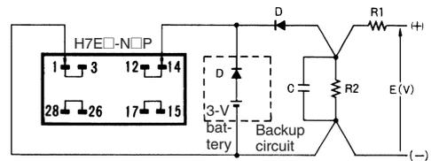
Use a diode (D) having a forward voltage as small as possible (0.1 V max. at  $I_F$  of 20 μA).
