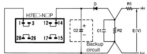
When a capacitor is used, its backup time can be calculated by the following formula:
