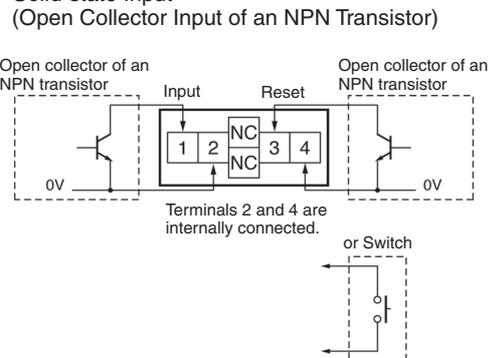
**Note:** 1. Residual voltage in the output section of Proximity Sensors or Photoelectric Sensors becomes less than 0.5 V because the current flowing from terminals 1 or 3 is as small as approx.  $10 \mu\text{A}$ , thus allowing easy connection.
