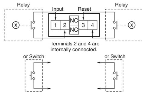
**Note:** Use Relays and Switches that have high contact reliability because the current flowing from terminals 1 or 3 is as small as approx.  $10 \mu\text{A}$ . It is recommended that OMRON's G3TA-IA/ID be used as the SSR.
