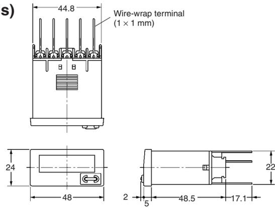
When using the Wire-wrap Terminal, be sure to use the correct wires and peripheral devices. (The correct wires, bits and sleeves are shown in the table on the right.)
