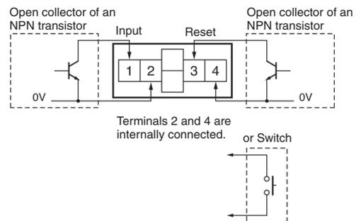
**Note: 1.** Residual voltage in the output section of Proximity Sensors or Photoelectric Sensors becomes less than 0.5 V because the current flowing from terminals 1 or 3 is small thus allowing easy connection.
