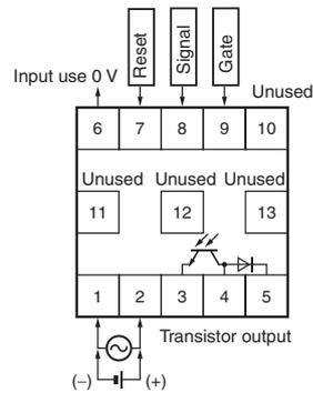
The power supply and input circuit are not insulated.
