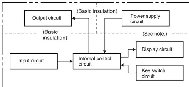
**Note:** Power circuit is not insulated from the input circuit, except for H5CX-A11/-A11S, which have basic insulation.
