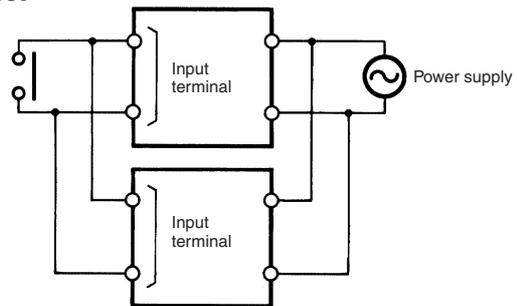
It is impossible to provide two independent power switches as shown below regardless of whether or not the Timers are different in phase.
