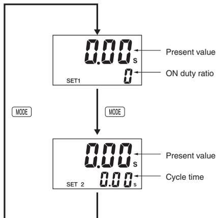
Set each digit for the ON duty ratio using the corresponding  $\uparrow$   $\downarrow$  keys. (The  $\uparrow$   $\downarrow$  keys for the 4th digit cannot be used.)
