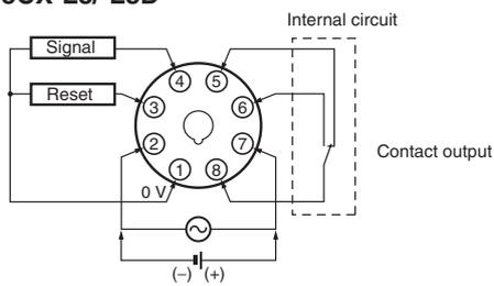
The power supply and input circuit are not insulated.
