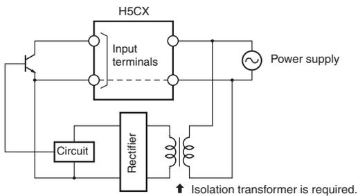
Make sure that the voltage is applied within the specified range, otherwise the internal elements of the Timer may be damaged.
