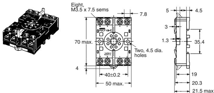
**Track Mounting/Front Connecting Socket**
