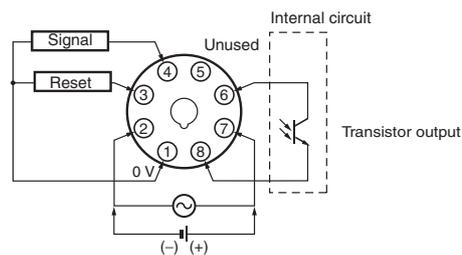
The power supply and input circuit are not insulated.
