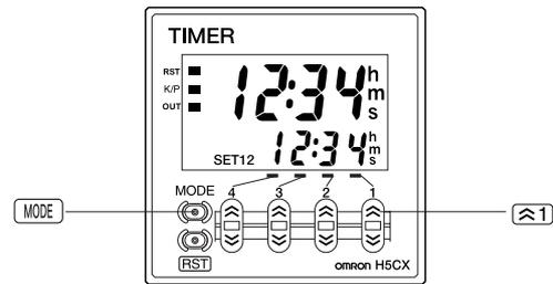
To change the mode to timer/twin timer selection mode, hold down the  $\text{F1}$  key for 1 s min. with the **MODE** key held down. The **MODE** key must be pressed before the  $\text{F1}$  key. If the  $\text{F1}$  key is pressed first, the mode will not change.
