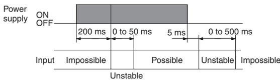
Turn the power ON and OFF using a relay with a rated capacity of 10 A minimum to prevent contact deterioration due to inrush current caused by turning the power ON and OFF.
