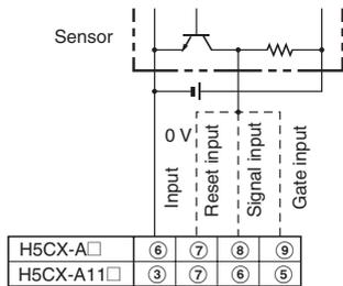
Operate with transistor OFF
