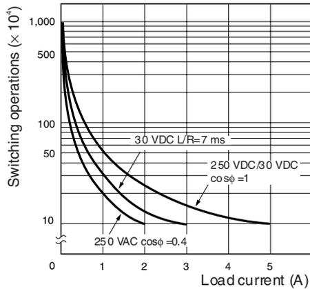
Reference: A maximum current of 0.15 A can be switched at 125 VDC (cosφ=1) and a maximum current of 0.1 A can be switched if L/R is 7 ms. In both cases, a life of 100,000 operations can be expected. The minimum applicable load is 10 mA at 5 VDC (failure level: P).
