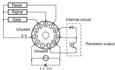
The power supply and input circuit of the H5CX-A11S have basic insulation.
