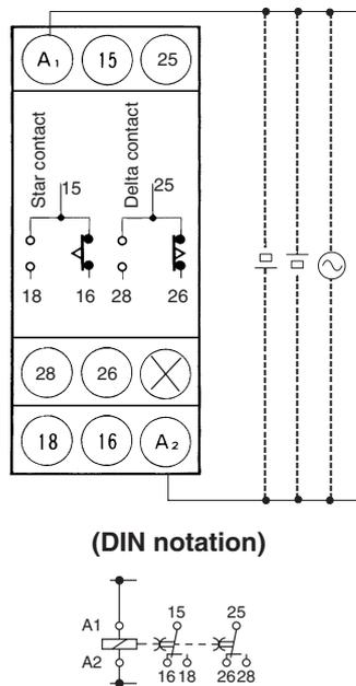
**Note:** DC supply voltage does not require the designation of polarity.
