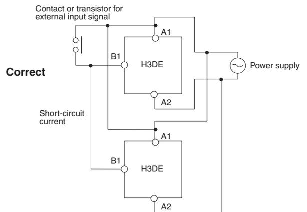
The H3DE Series is provided with a transformerless power supply system.
