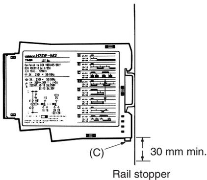
The H3DE can be mounted and dismantled with ease if a distance of 30 mm or more is kept between the H3DE and the top surface of other equipment located below the H3DE.
