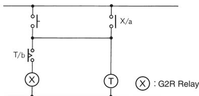
In the case of the above circuit, the H3RN will be in pulse operation. Therefore, if the circuit shown on page 3 is used, no auxiliary relay will be required.
