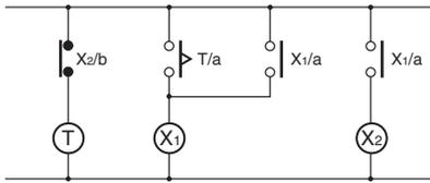
⊗ : Auxiliary relay such as G2R Relay
