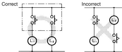
Use the following safety circuit when building a self-holding circuit with the H3RN and an auxiliary relay, such as a G2R Relay, in combination.
