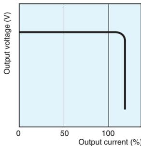
**Note:** Do not allow the short-circuited or overcurrent state to continue for more than 20 s, otherwise it may damage the element.
