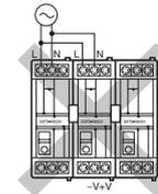
Do not cross-wire Blocks or wire between a Block and another device. If the rated current is exceeded, Bus Line Connectors may be damaged.
