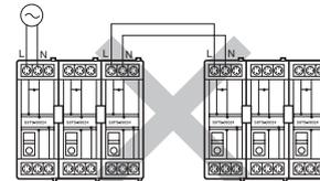
When Basic Blocks are linked together, it is necessary to wire the GR terminal of only one Block, not all the Blocks.
