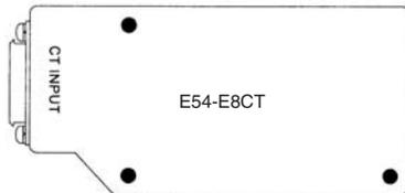
Use this CT input unit in combination with the E53-E8Q voltage output unit.
